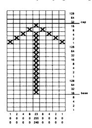
Now you've seen how to design a character by placing dots on a grid and translating the dots to decimal equivalents. The last step in defining a character is to send this information to the printer.
